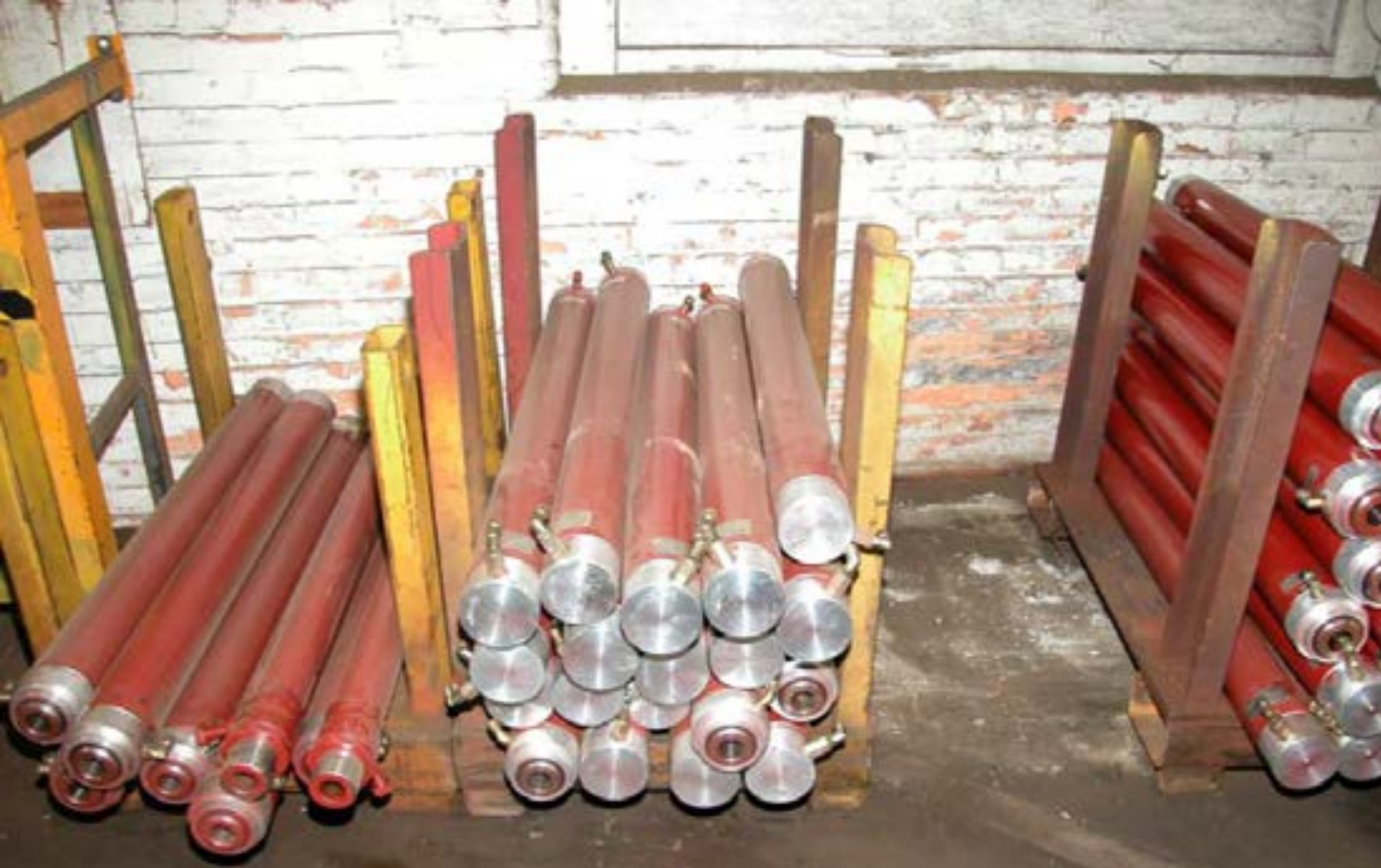
Completed hydraulic cylinders
