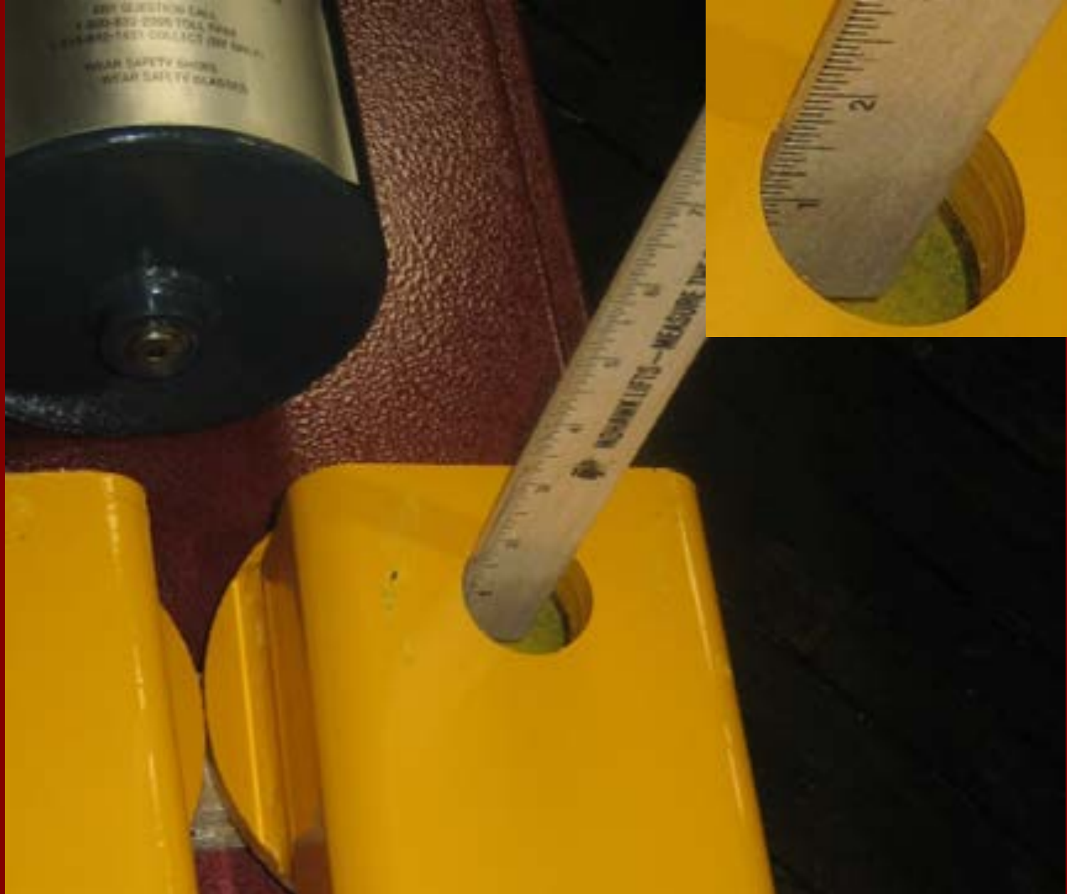
This picture shows reinforced section of each swing arm for maximum support.
