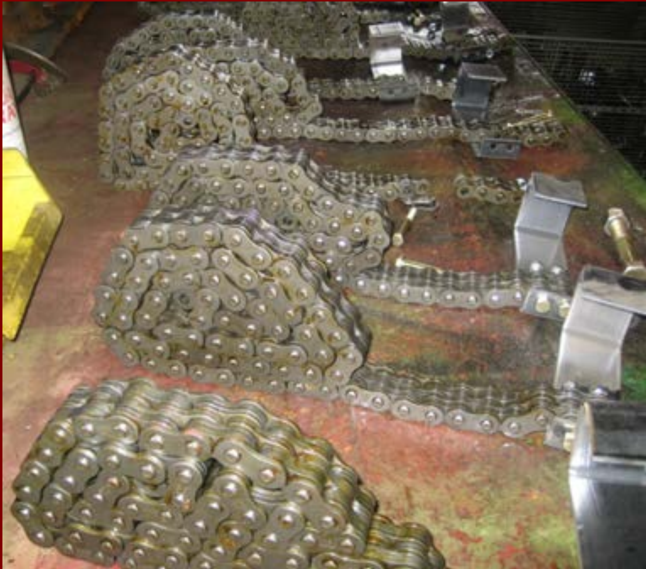
A-7 and System I #646 leaf chain prior to installation in the carriages.
