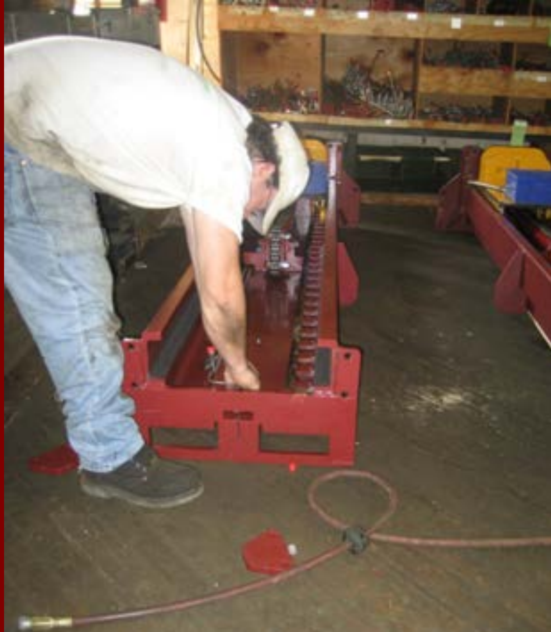
Assembling internal hydraulic bulk-head fittings.
