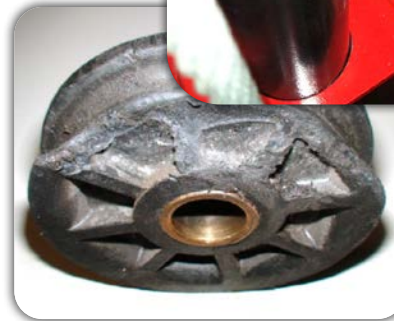
Broken Plastic Cable Roller
