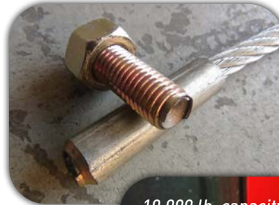
Broken, Low-Grade Cable Bolt
