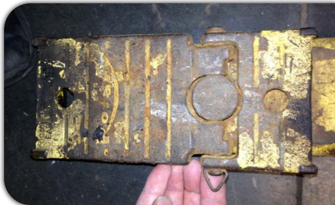
Shows broken pin & ability of flip up adaptor to come apart. Note pin backing out of flip pad.
