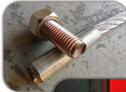
Broken, Low-Grade Cable Bolt
