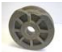
WORN CABLE ROLLER
