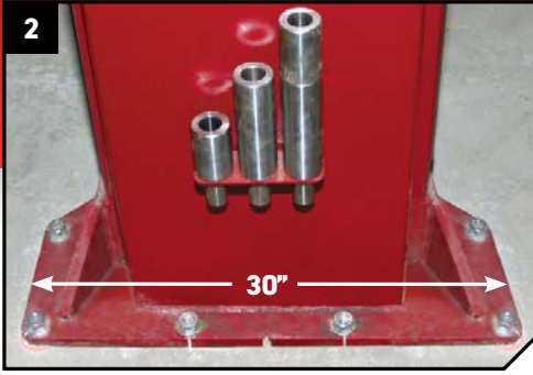
▲ Mohawk's large and stable footprint measures 30" wide and is made of 3/4" thick plate. Mohawk's large base with 8 lag bolts gives stability to the lift, while distributing the load to the shop floor.
