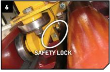
**All position** mechanical locks in both columns engage the full length of travel
