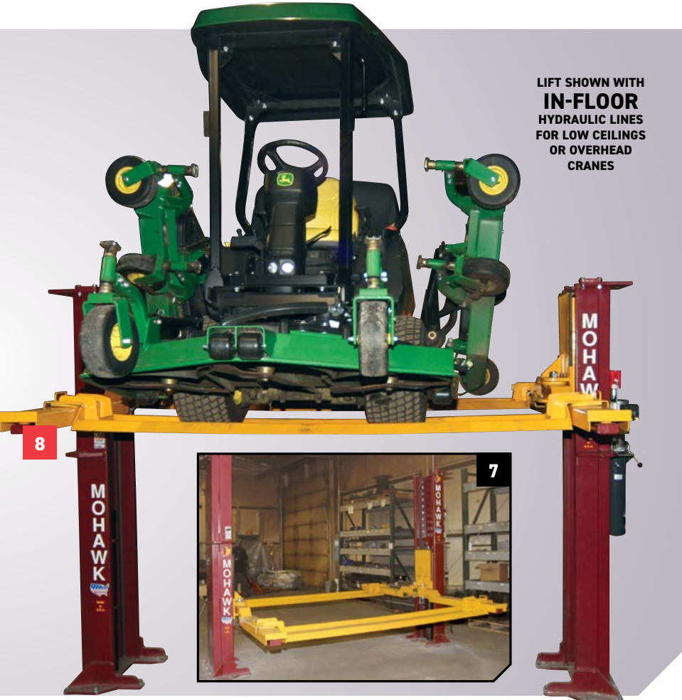
▲ Mohawk's large and stable footprint measures 30" wide and is made of 3/4" thick plate. Mohawk's large base with 8 lag bolts gives stability to the lift, while distributing the load to the shop floor.
