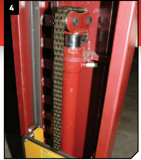
▲ Heavy duty post design using DUAL cylinders with #646 leaf chain lifting or direct drive over DUAL bearings
