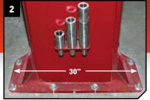
Mohawk's large and stable footprint measures 30" wide and is made of ¾" thick plate. Mohawk's large base with 8 lag bolts gives stability to the lift, while distributing the load to the shop floor.
