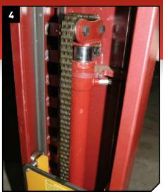
Heavy duty post design using DUAL cylinders with #646 leaf chain lifting or direct drive over **DUAL** bearings
