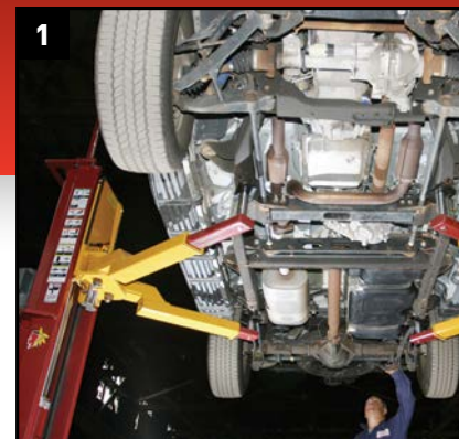
▲ Two post lifts offer FULL under vehicle access for repairs, takes up minimal bay space, while leaving vehicle hanging free for tire, brake or any other need.
