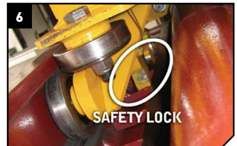
▲ All position mechanical locks in both columns engage the full length of travel.
