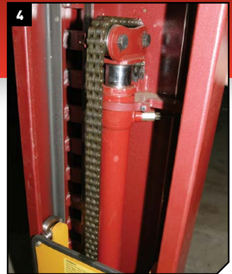
▲ Heavy duty post design using DUAL cylinders with #646 leaf chain lifting, over DUAL bearings.
