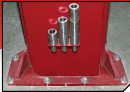
▲ Mohawk's large and stable footprint measures 30" wide and is made of 3/4" thick plate. Mohawk's large base with 8 lag bolts gives stability to the lift, while distributing the load to the shop floor.
