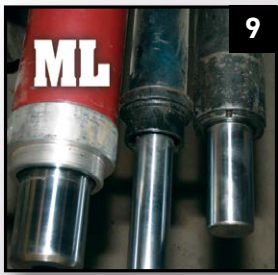
9 ▲ LARGE 4" CYLINDERS equal longer seal life and lower operating pressures vs. smaller competitive cylinders.
