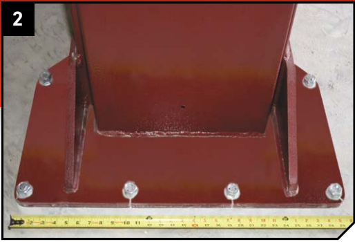
2 ▲ Mohawk's large and stable footprint measures 30" wide by 24" is made of 3/4" thick plate. Mohawk's large base gives stability to the lift, while distributing the load to the shop floor.
