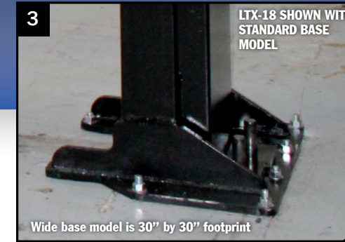
▲ LiftPoint's large and stable footprint measures 30" wide by 24" and is made of 1/4" thick plate. LiftPoint's large base gives stability to the lift, while distributing the load to the shop floor.
