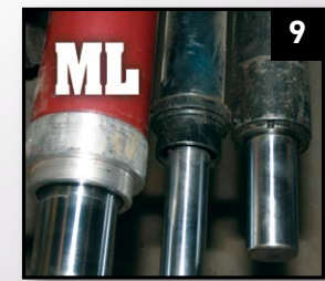
9 ▲ LARGE 4" CYLINDERS equal longer seal life and lower operating pressures vs. smaller competitive cylinders.
