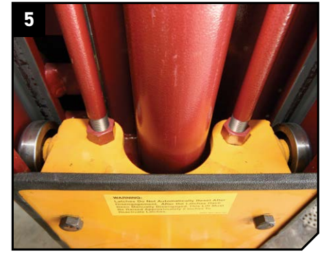
5 ▲ Each carriage rolls on (8) 4" double sealed, self lubricating, heavy duty ball bearing rollers for a lifetime of trouble-free service (not plastic slide blocks).
