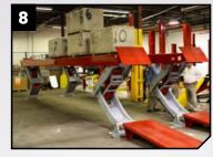
▲ Mohawk uses a patented volumetric fluid powered system to ensure the lift starts level and stay level...both front to rear & side to side. Shown with a 25% offset load.
