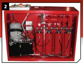
▲ Patented Hydro-Mechanical synchronization with electrical backup safety. Mechanical Torsion Bar prohibits master/slave cylinders (8 total) from moving at differential speeds. ZERO Equalization/Fault Codes to maximize uptime, and minimize service/parts/repair.
