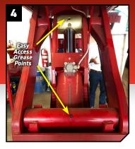
▲ Mohawk VRL uses a vertical cylinder design with a short stroke - meaning less wear of the piston/ram system.
