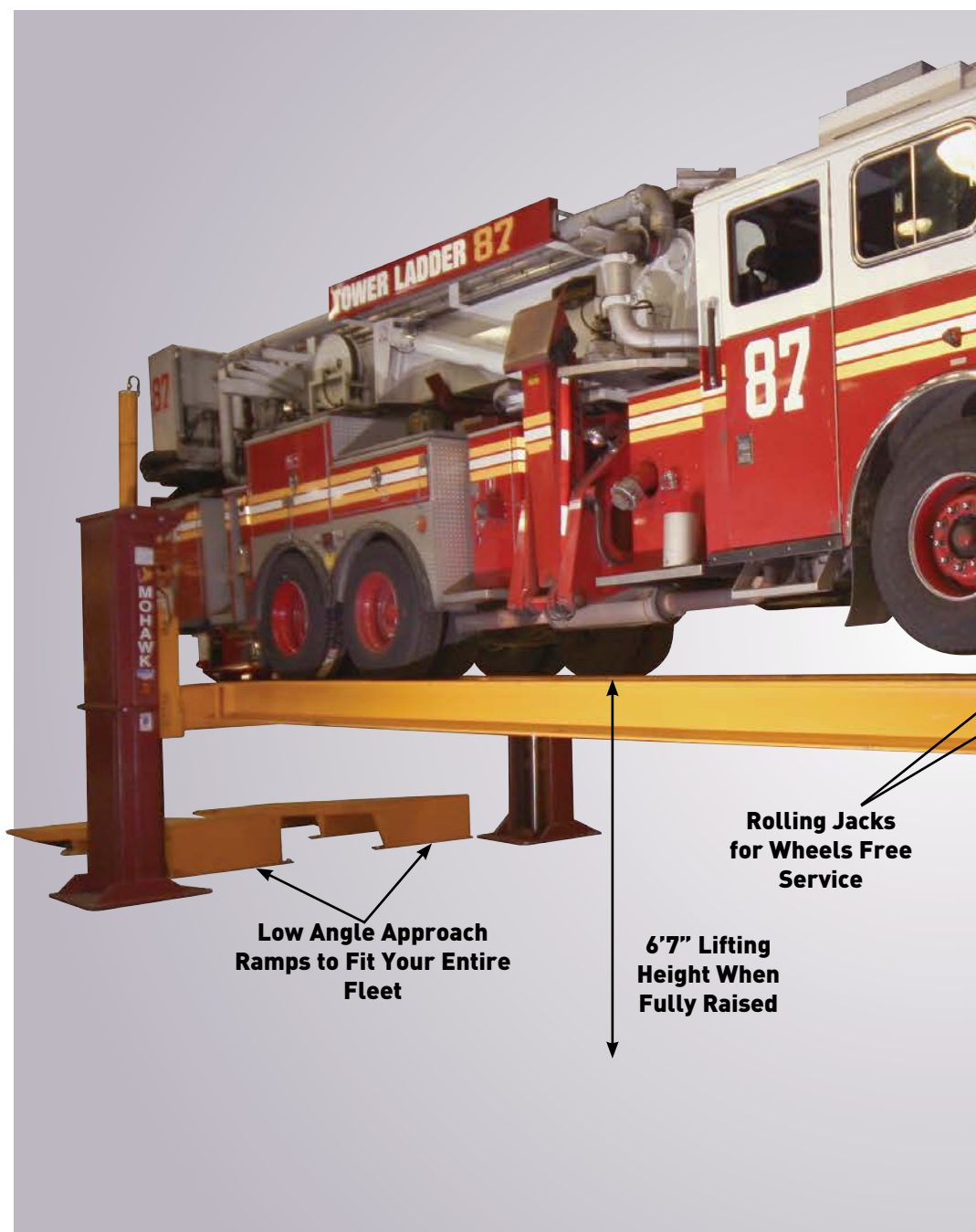
▲ Lifting Columns built of 1" by 7" Fork Lift mast section with all carriages riding on 5" sealed rollers. Inverted heavy duty lifting cylinders in each column; uses no chains or cables to wear or which need replacing.
