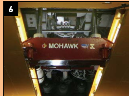
ROLLING JACKS & TRACK LIGHTING Optional electric/ hydraulic rolling jacks for wheel free service, or florescent lighting to illuminate vehicle undercarriage
