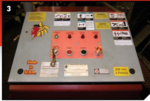
▲ Control box is positioned where you want it. Simple control system of up, down and park (lock) for assuring all locks are resting on the safeties.
