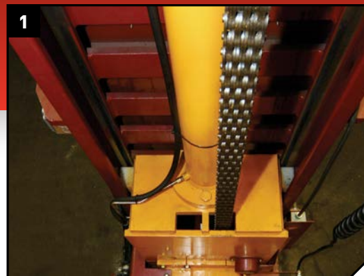
▲ Lifting Columns built of 1" by 7" Fork Lift mast section with all carriages riding on 5" sealed rollers. Inverted heavy duty lifting cylinders in each column; uses no chains or cables to wear or which need replacing.
