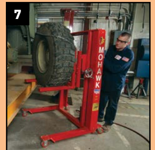
TIRE DOLLY Optional 1000 or 2000 lb. capacity tire dolly to remove the largest of wheel assemblies
