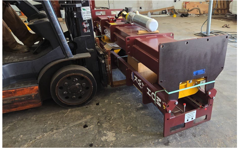
SIDE LOADING POSITION, BE SURE TO BALANCE LOAD DURING TRANSPORT.
