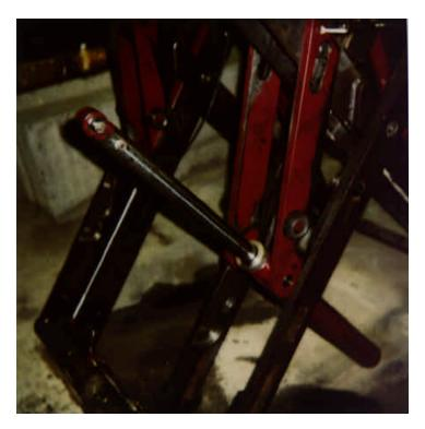
11. HOLD CYLINDER FIRMLY AND PRESS SIDE SUPPORT ARMS AWAY FROM CYLINDER (ENSURE THAT C-CLAMP IS STILL SECURE). REMOVE CYLINDER. SEE BELOW.
