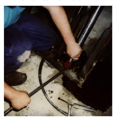
$10.\,$  ONCE ROD IS FREE OF MAIN TUBE, PIVOT CYLINDER SO ROD IS POINTING UP. SEE BELOW.
