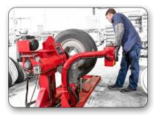
**TCX625HD Tire Changer** Service over-the-road truck tires safely and easily. Easy-to-use features make it ideal for match-mounting.
