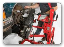
AutoComp Elite™ On-Car Brake Lathe
