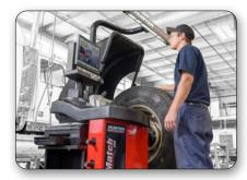
ForceMatch® HD Balancer End wheel vibrations for a wide range of vehicles from passenger cars to Class 8 trucks.
