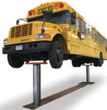
are the dominant drive system, your choice in lifts is of two; single cylinder or twin cylinder. Twin cylinder is the more common lift based on reliability. Of the drive mechanisms offered, the size of the of the cylinder(s) is important as larger cylinders work under less pressure, making the seals last longer and hydraulic pump work easier. On the downside, a larger cylinder is slower to fill with fluid, yet most lifts still raise in about 45 seconds.
