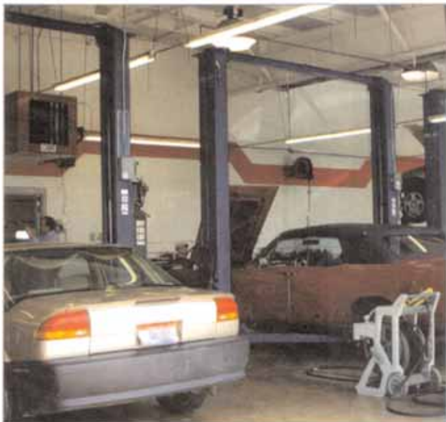
The lift area should be kept free of grease, oil, tools, equipment, trash and other items that could interfere with the operation of the lift or with the technician using the lift.
